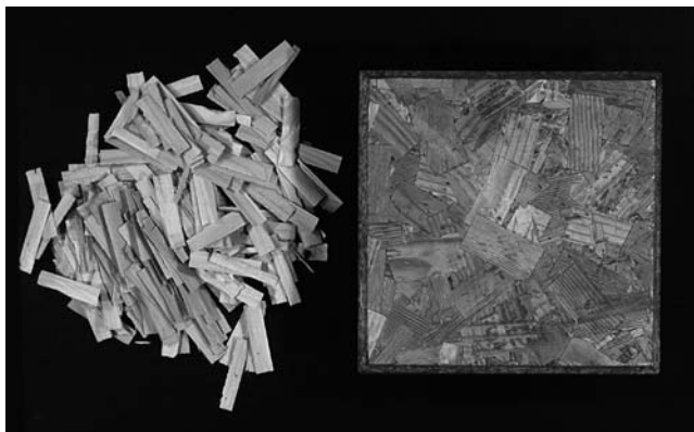
FIGURE 10.9 Flakes used to make flakeboard.
