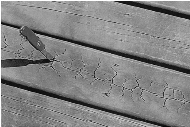
FIGURE 7.5 Cross-grain checking in juvenile wood.
