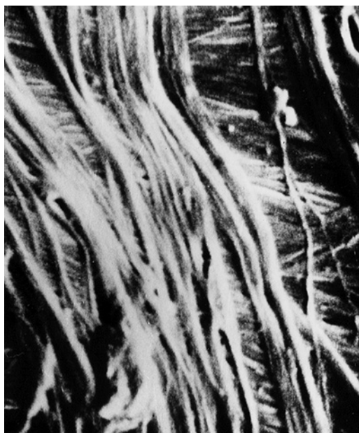
FIGURE 11.10 Scanning electron micrograph of delignified softwood fiber wall ( \times 16,000 ).
