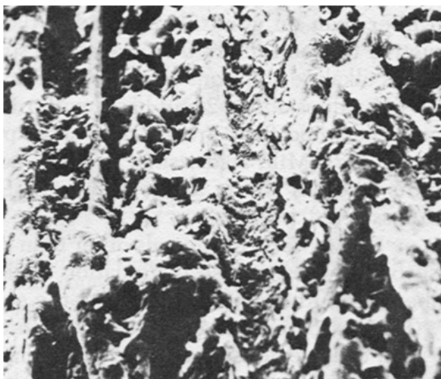
FIGURE 11.18 Scanning electron micrograph of sodium chloride in southern pine cell (×400).
