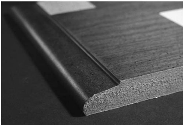
FIGURE 10.11 Thin veneer over medium-density fiberboard.
