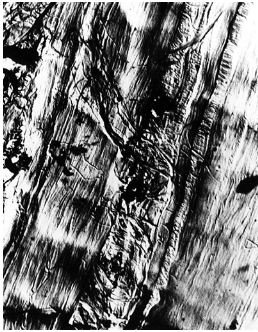
FIGURE 11.9 Scanning electron micrograph of softwood fibers embedded in lignin ( \times 400 ).
