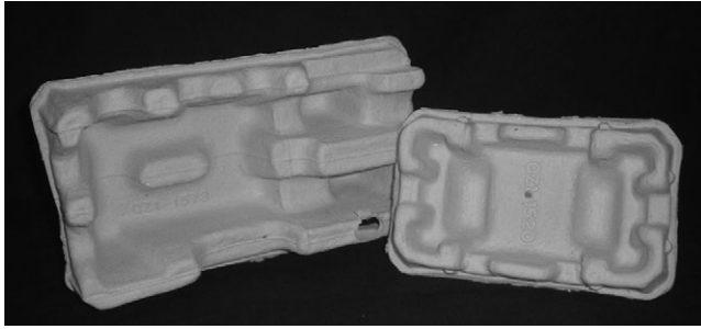
FIGURE 12.5 Products made by pulp molding.
